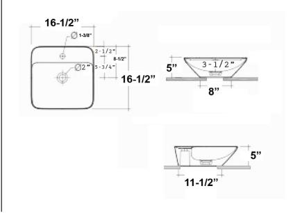
Dimensions of fixture are nominal and may vary within the range of tolerances established by AMSE Standard A112.19.2.2018 Dimensions and specifications subject to change without notice.
